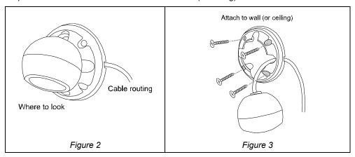
Step4: Put together the bracket and the lens, and slightly adjust the camera lens. Make sure it faces your target surveillance area.
